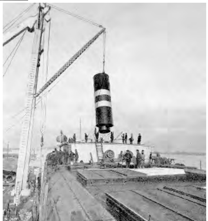
Placing stack on John J. Boland - Ecorse yard [GLEW BKLt]
